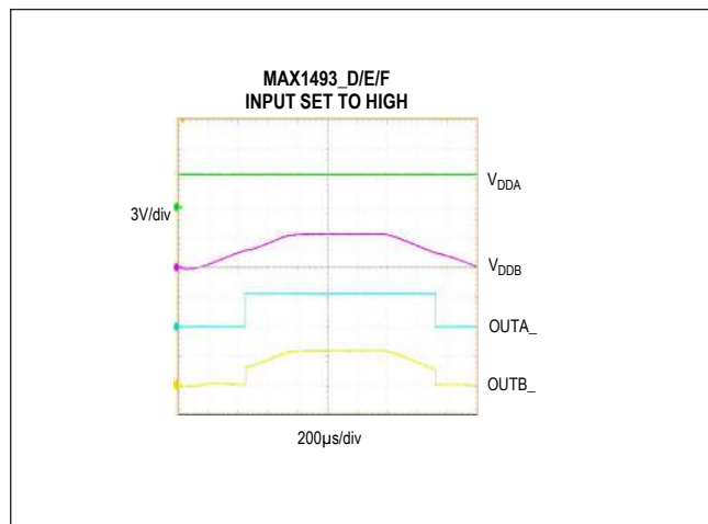
Figure 6. Undervoltage Lockout Behavior (MAX1493_D/E/F High)
