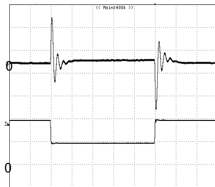
Figure 9: Output voltage response to step-change in load current (75%-50%-75% of Io, max; di/dt = 1.0A/μs). Load cap: 100μF tantalum capacitor and 1μF ceramic capacitor. Top Trace: Vout (100mV/div, 200us/div), Bottom Trace: Iout (10A/div). Scope measurement should be made using a BNC cable (length shorter than 20 inches). Position the load between 51 mm to 76 mm (2 inches to 3 inches) from the module
