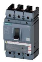
circuit breaker 3VA5 UL frame 250 breaking capacity class M 35kA @ 480 V 3-pole, line protection TM230, FTAM, In=200A overload protection Ir=200A fixed short-circuit protection Ii=5...10 x In UL 489 SB (naval), 50° C without connection
