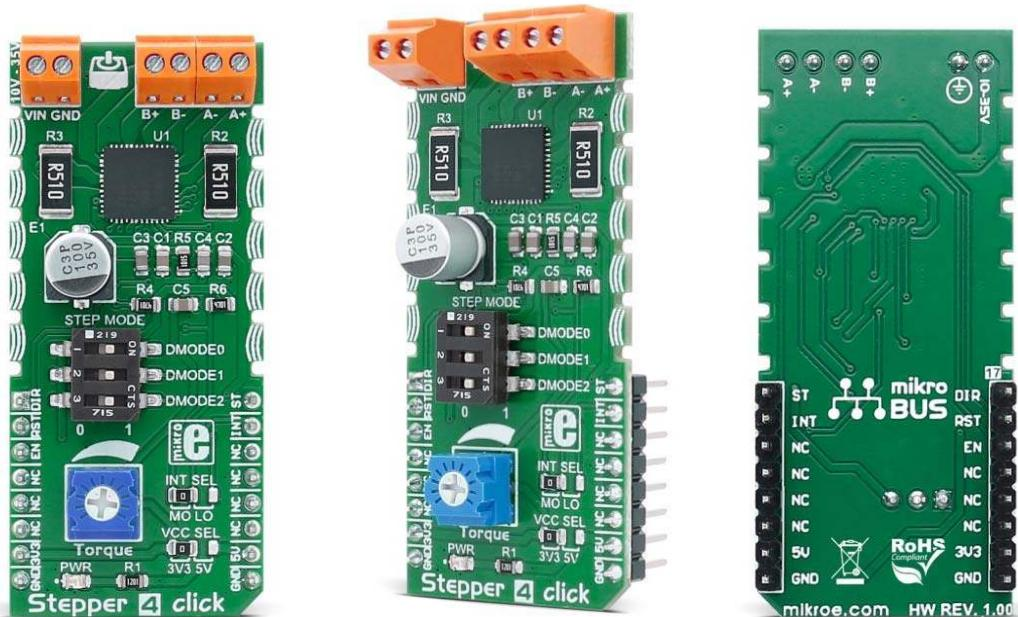
**Stepper 4 click** can be used for driving a stepper motor and controlling its step resolution, rotation direction, and time between the steps. It has output drive capability of **2A**.
