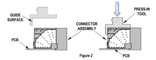
3. Using the application tool and an appropriate press, seat the Orthogonal Direct Ram module until there is less than 0.10mm (.004 in) clearance between the bottom of the plastic housing and the surface of the PCB. See Figure 3.
