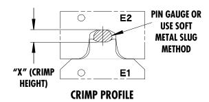
Use gauge pins or soft metal slug (solder) method to measure the "X" dimension. Verify tooling crimp height calibration by referring to the Go/No Go dimensions shown in the chart below.
