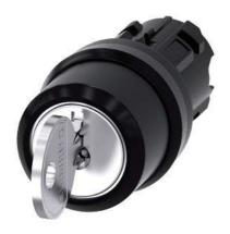
RONIS key-operated switch, 22 mm, round, plastic, lock number SB30, with 2 keys, 3 switch positions I-O-II, latching, actuating angle 2x45°, 10:30h/12h/13:30h, Key removal II, possible special locks: SB31, 421, 455, with laser labeling, upper case and lower case, always upper case at the beginning of the word
