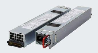
Advanced Energy's Artesyn DS1100SLPE series bulk front end AC-DC power supply accepts a wide range 90–264 Vac input and provides a main 12 V output plus a 3.3 V standby output. Rated at 1,100 watts it is an 80 Plus Platinum supply with a high peak efficiency of 94%. Housed in an industry standard 1U x 2.1 inch rack-mounting package, the power supply is ideal for space-constrained applications. This series comes in two airflow versions – dc-connector to ac-connector and vice versa.
