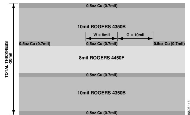
Figure 19. Evaluation Board Cross Sectional View
