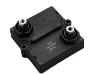
Ohmite's TAP800 Series dissipates 800 watts of power when used with a liquid or air cooled heat sink system. The Ohmite CP4 (https://www.ohmite.com/cp4-series-chillplate/) is an example of properly designed heat sink. The TAP800 compliments the 600 watt (TAP600), 650 watt (TAP650) and 2000 watt (TAP2000) product offerings. Applications include variable speed drives, power supplies, robotics, motor control, control devices, and other power designs.
