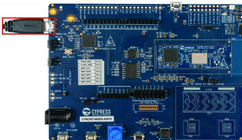
Figure 2-5. Connect USB Cable to USB Connector on the Board
