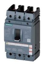
molded case switch 3VA5 UL frame 250 max. sh-circ breaking capacity 65kA @ 480V 2-pole, line protection MCS110, In=150A without overload protection self-protection li=16 x In without connection
