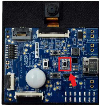
Figure 8: SLN-VIZN-IOT Manual Registration Button
