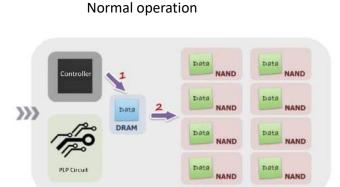
The SSD is powered by the host power, and the power loss protection circuit is charged by the host power. Unexpected Power Loss happens
