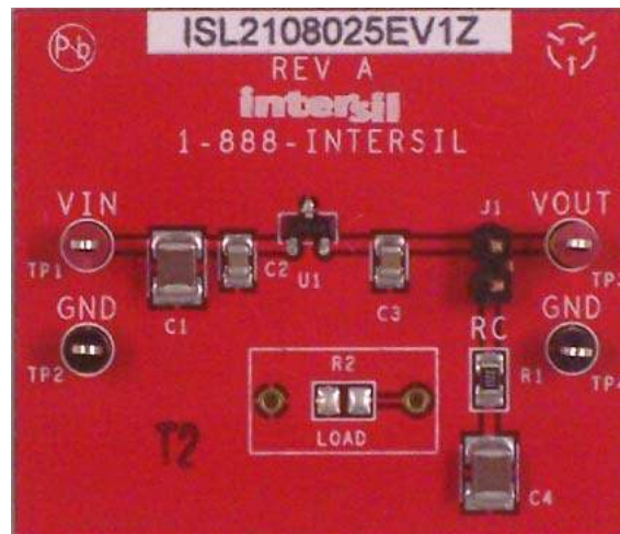
FIGURE 1. VOLTAGE REFERENCE EVALUATION BOARD (ISL2108025EV1Z)
