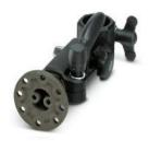
140.5 mm housing attachment, for max. load 10 kg, with ball joint and fastening plate 60 mm, pivotable in 15 $^{\circ}$  increments, for 30 mm wall/profile bracket, material: black glass-fiber reinforced polycarbonate PC, and black anodized aluminum, 342 g
