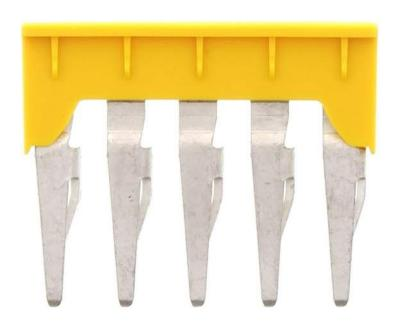
Insulated cross-connector, No. of poles: 5, Mounting type: Plug in, Width: 31.9 mm, Rated cross-section: 6 mm², Colour: Yellow
