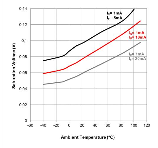
Testcondition: I<sub>E</sub>= 5mA, Normalized to 25°C
