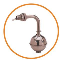
The SSF29 type is a side mount vertical switch designed to give reliable switching at higher pressures, up to 40 bar. The switch is mounted in the side of the tank, from the inside, so requires access to the inside of the tank.
