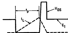
Fig. 2 - Clamped Inductive Waveforms
