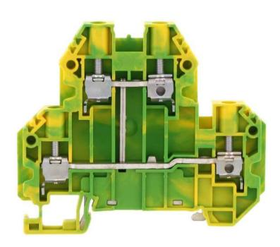
Protective-earth double-level terminal, Screw connection, Mounting type: Mounting rail TS 35/7.5, Rated cross-section: 4 mm², Width: 6.1 mm, Colour: Green-yellow
