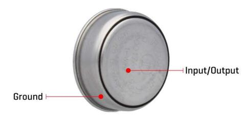
The device is capable of powering itself up through the data line by employing the so-called parasite power supply. Parasite PSU contains an internal capacitor, which provides enough current for the proper operation, once it has been charged by the data line. To allow proper functioning of the parasitic PSU, the idle state of the data line is HIGH, while the data line of the DS1990A is in an open-drain configuration, pulling the data line to a LOW logic level when asserted.
