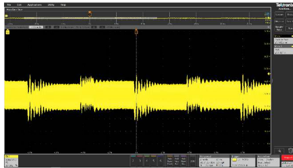
Figure 25. Transient Load on 9 V BUS
