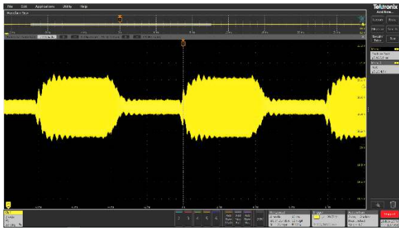
Figure 28. Transient Load on 20 V BUS
