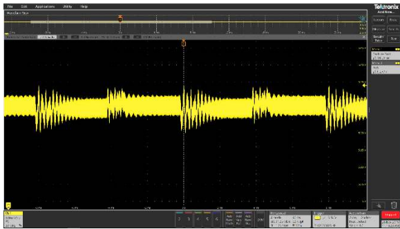
Figure 24. Transient Load on 5 V BUS
