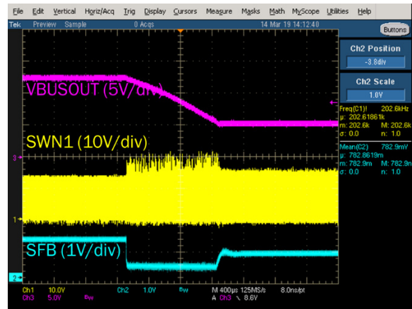
Figure 17. 12 V to 5 V Transition with No Load
