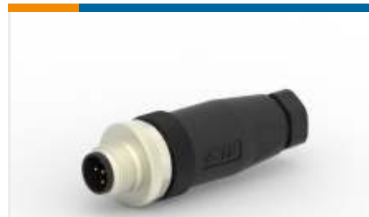
TE Part #T4111401051-000 M12,MALE,STRAIGHT,B CODE,5P, PG7,GOLD
