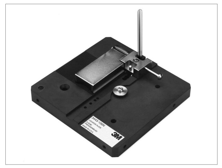
The 3M Locator Plate 3443-106N is designed to aid in the assembly of the preassembled and two-piece  $3M^{TM}$  Delta Connector and pin 9 through 37 position connectors. End-to-end, as well as daisy chain assemblies, can be made. Set-up and assembly instructions are based on termination procedures with the 3M manual and pneumatic presses.
