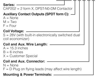
D = 2X M5 Bottom Mount with 4X, M6 x 1 Female thread terminals
