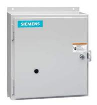
Mechanically held lighting contactor, Contactor amp rating 60Amp 0NC \_ 8NO poles, 440VAC 50HZ/480VAC 60HZ coil, Non-combination type, Enclosure NEMA type 1, Indoor general purpose use
