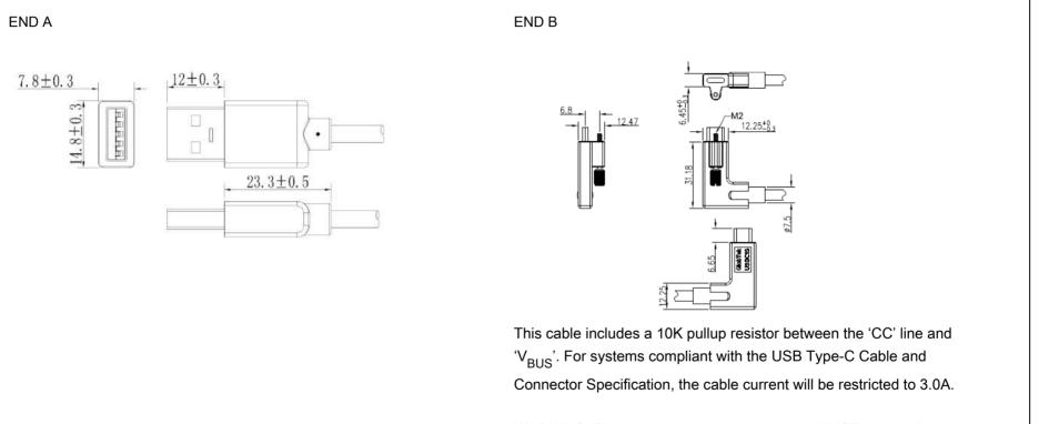
WARNING: The power supply's current rating MUST be  $\geq$ 3.0A to prevent permanent equipment damage and overheating which may result in fire.
