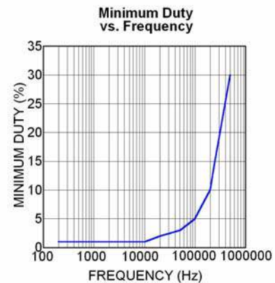
Figure 5. Minimum Duty Cycle for Varying PWM Frequency
