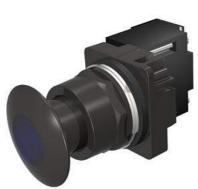
30mm BlackMax, Epoxy Coated Corrosion Resistant Complete Metal Unit Illuminated Push-Pull Operator Full Voltage, 24V AC/DC Incandescent Lamp Mushroom Head Cap Small 1 3/4" (44.5 mm) Metal, Black with Blue Lens 3 Position Momentary UL Listed, CSA Certified NEMA 1,3,3R,4,4X,12,13 & Automotive Standards
