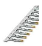
Crimp contact, Socket, rolled, Taped articles, number of pieces per reel: 10000, contact diameter: 1 mm, crimp range:  $0.22~\text{mm}^2$  ...  $0.56~\text{mm}^2$ , Item is lead-free in accordance with RoHS II without Exemption 6c (Pb <0.1%)
