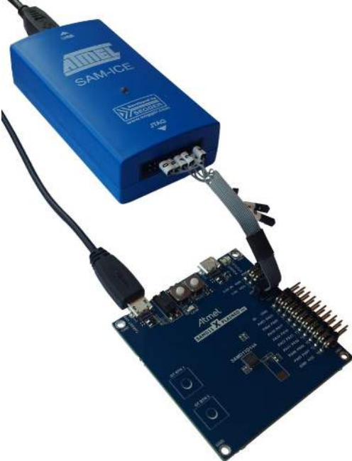
Figure 7-2. SAM-ICE using an Atmel-ICE Adapter
