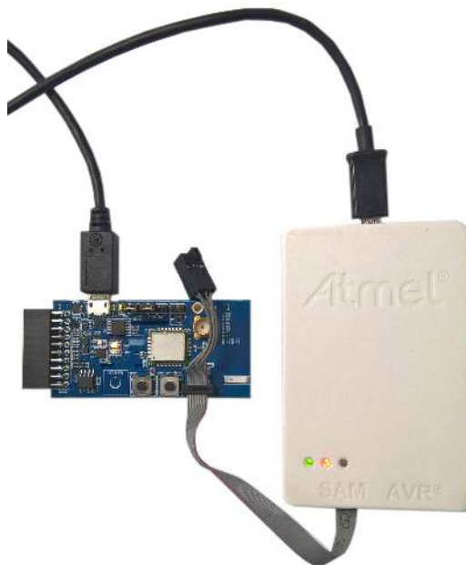
Figure 2-9. Connecting Programmer/Debugger with SAMR30 Module XPro Extension Board
