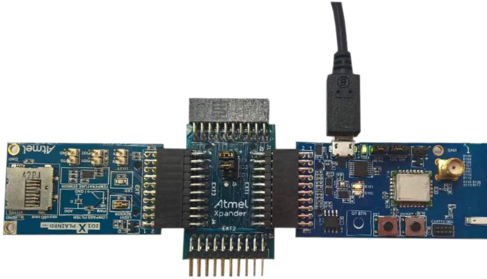
Figure 2-2. SAMR30 Module XPro Interfaced with Standard XPro Extension Board
