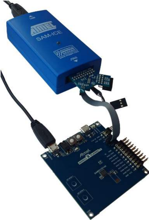
Figure 7-2. SAM-ICE using an Atmel-ICE Adapter
