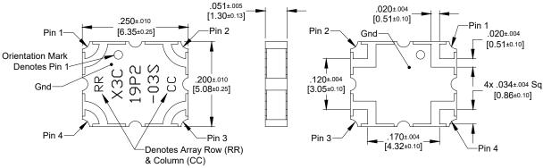
Dimensions are in Inches [Millimeters] X3C19P2-03SS Mechanical Outline
