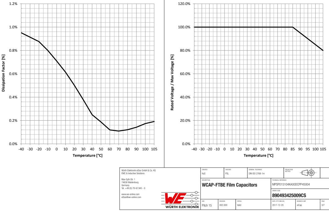
**Rated Voltage vs. Temperature:**
