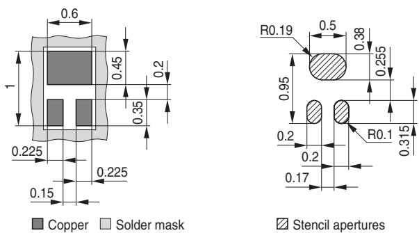
■ Copper   □ Solder mask   □ Stencil apertures
