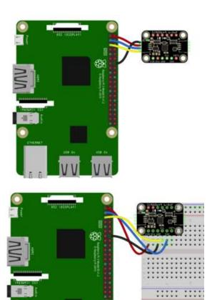
Pi 3V to sensor VCC (red wire)
