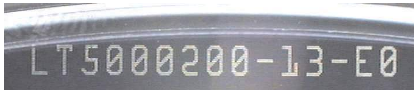
Figure 3-2. Wafer Identification Code 1
