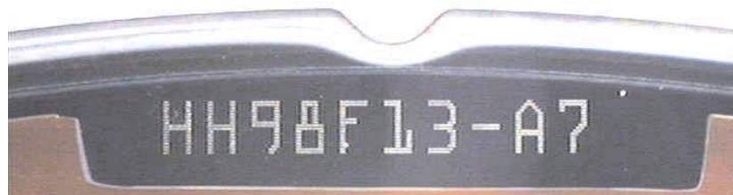
Figure 3-3. Wafer Identification Code 2
