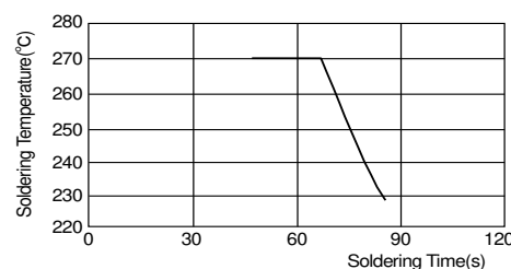
[Allowable Reflow Soldering Temperature and Time]
