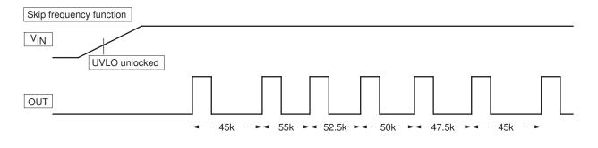
Switching frequency is changed as follows.  $\dots \times 0.9 \rightarrow \times 1.1 \rightarrow \times 1.05 \rightarrow \times 1 \rightarrow \times 0.95 \rightarrow \times 0.9 \rightarrow \times 1.1 \dots$ It's repeated by this loop.
