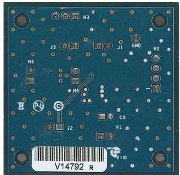
Figure 2. SSM2375 Evaluation Board Bottom View
