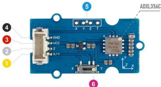
**④ GND:** connect this module to the system GND
