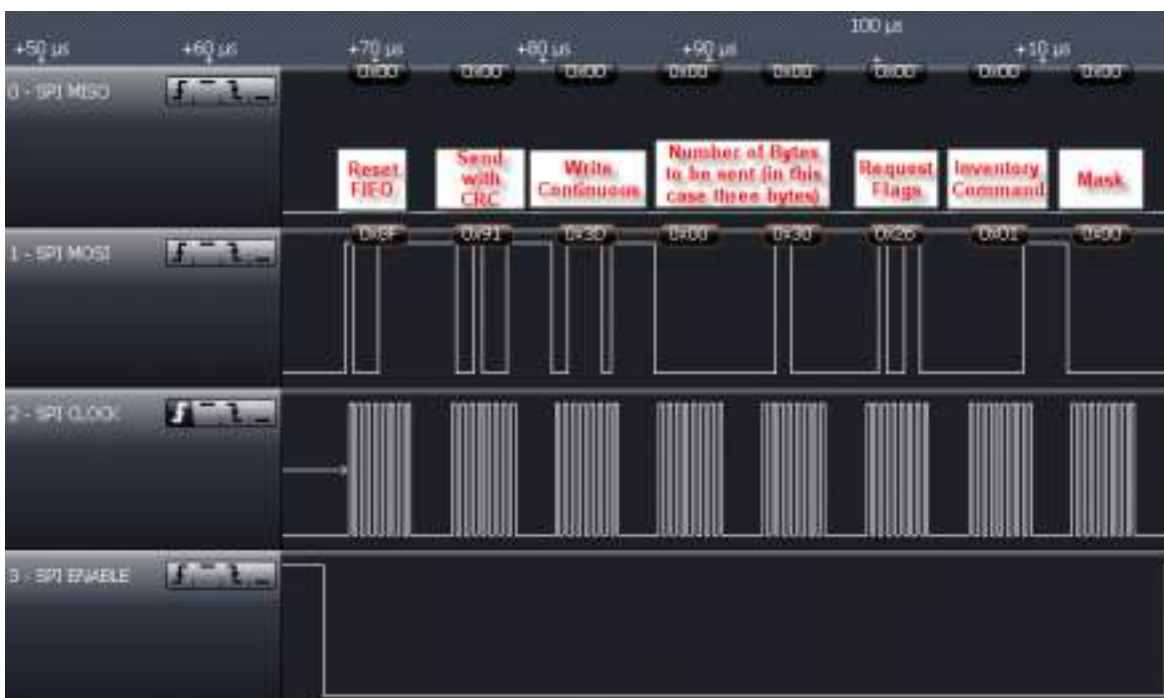
Figure 6-22. Inventory Command Sent From MCU to TRF7970A
