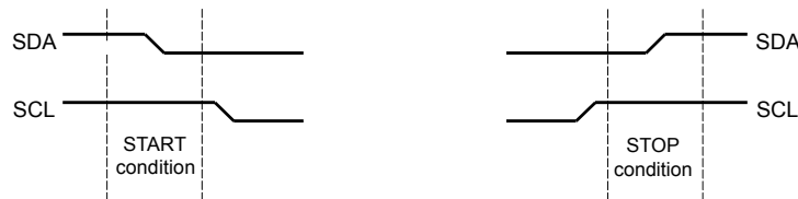
Figure 15-3. START and STOP Conditions
