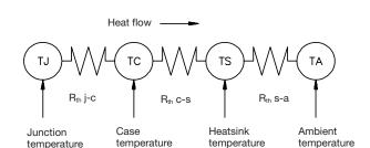
Thermal resistance: R<sub>th</sub> j-c = junction to case
