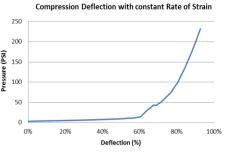
\*Specimen Area: 1inch<sup>2</sup> Rate of strain= 1.0mm/min
