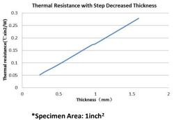
The thickness of sample is controled by limit slice Decreased Thickness step = 0.1mm
