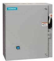
Non-reversing motor starter, Size 3, Three phase full voltage, Solid-state overload relay, OLRelay amp range 25-100A, 208VAC 60HZ coil, Combination type, 100A non-fusible disconnect, Enclosure NEMA type 1, Indoor general purpose use, Standard width enclosure
