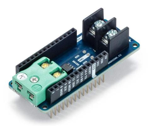
The MKR THERM Shield allows a board of the MKR family to acquire temperatures from a thermocouple of type K and a DS18Bxx digital one wire sensor. The Thermocouple is a kind of temperature sensor that offers high accuracy and a wide range of measured temperatures. Its analog nature requires specific interfacing and this shield relies on the MAX31855 thermocouple digital interface.
