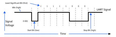
You can configure the UART baud rate, parity, and stop bits settings on the device with the **BD**, **NB**, and **SB** commands respectively. For more information, see <u>Serial interfacing commands</u>.
