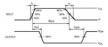
Note 1: Pulse Width 50  $\mu$ s, Duty Cycle 10% Output Impedance 50  $\Omega$ ,  $t_f \le 5$ ns,  $t_f \le 10$  ns
