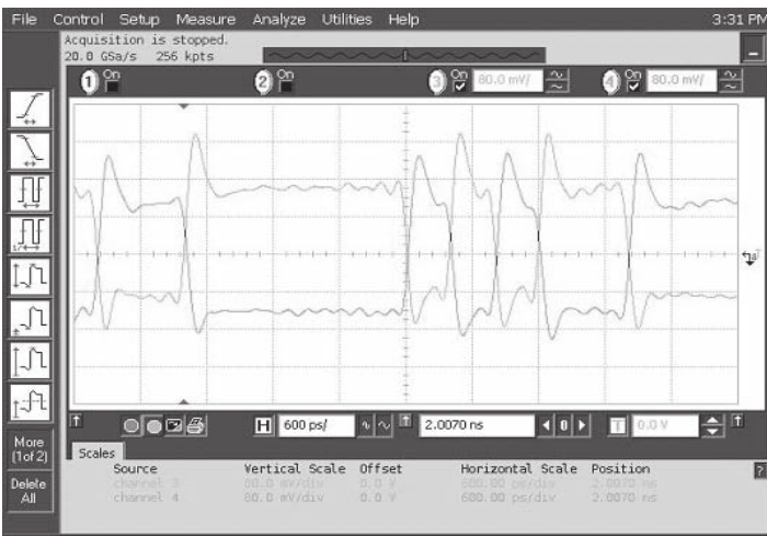
Data Waveforms, 2.5Gbps (left) & 5.0Gbps (right)
