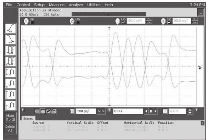
Data Waveforms, 2.5Gbps (left) & 5.0Gbps (right)
